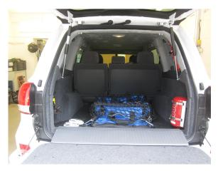
What is required is a dedicated rear cargo design that incorporates suitably rated shackle points, appropriate containers and netting to provide restraint for tools and first aid kits etc. In addition, suitably rated brackets are needed for all items bolted to the vehicle's internal wall e.g. fire suppression tanks and wheel jack.
