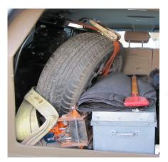
Some time ago a client asked me to conduct a safety review of this vehicle (left), which was operating in a very hostile environment. It is unfortunately a good example of a very unsafe vehicle. Without too much effort, the unrestrained, and poorly restrained, equipment will end up flying forward in the vehicle cabin and will quite likely cause serious injury to the occupants.
